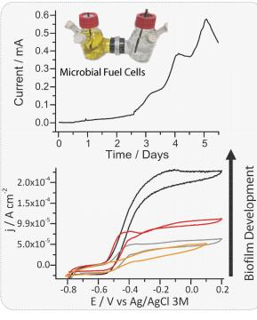
Attaching biofilms of **exoelectrogenic bacteria** to conductive surfaces allows us to couple their metabolism to electricity generation. These bacteria **effectively 'eat' toxic metals to produce electricity and biosynthesise nanoparticles in the process!**
